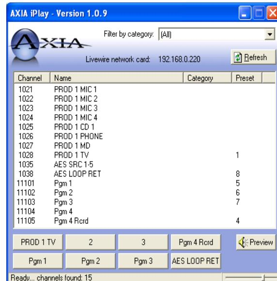
Figure 1-8: iPlay with ACL in effect
